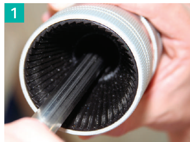
CUT AND DEBURR PIPE
